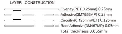
**Tactile:** The most conventional structure of the membrane switch. Usually the panel is embossed. The domes of different forces are installed under the panel to obtain a good tactile feedback.
